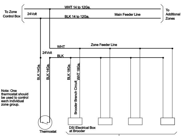
This schematic represents a group of four (4) brooders controlled by one (1) thermostat. Additional zones should be wired as shown.
