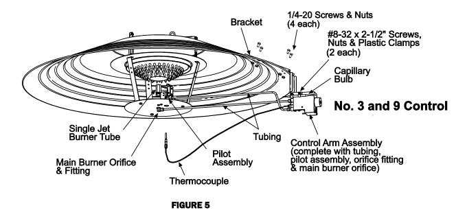
2. Place the bracket for the gas control arm over the canopy and secure using four (4) ½-20 screws, washers and nuts from the fastener kit. See Figures 5 and 5a. NOTE: Mounting the control bracket to a 34" canopy requires use of the set of holes located at the end portion of the control bracket only. See Figure 7. Attach the gas valve to the control arm bracket using the fasteners indicated above and below for the 2B, 3 and 9 controls.
