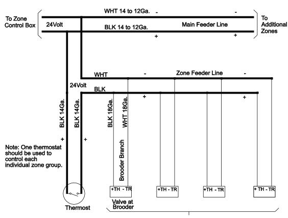
This schematic represents a group of four (4) brooders controlled by one (1) thermostat. Additional zones should be wired per this schematic to maintain correct polarity for DC operation.
