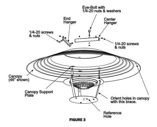
2. Assemble the end and center hangers to the support braces using five (5) ½-20 screws and nuts from the fastener kit. Assemble the eyebolt to the center hanger using two (2) ½-20 nuts and washers. See Figures 3 and 4.
