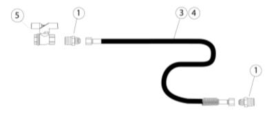
G) Manual Gas Shut-Off Ball Valve - 1/2"NPT, Part #30285000
